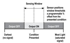
Output ON and OFF conditions can be reversed using the LO/DO switch.
